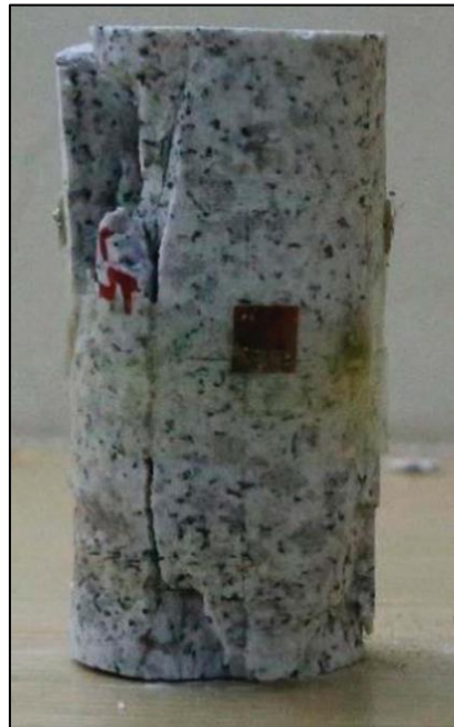
Figure 2 Granite specimen after failure [1]
